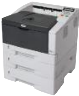
FS-1370DN shown with 2 additional paper feeders for an 800 sheet paper capacity
